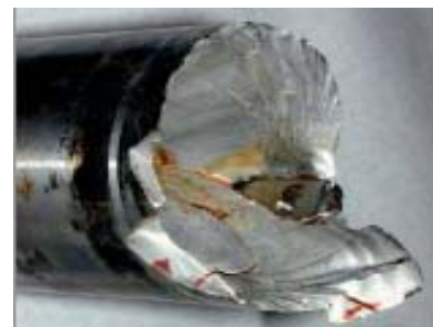
Pump Shaft Fatigue Failure.
