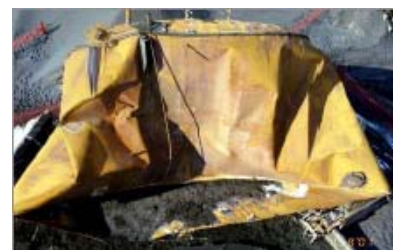
Collapsed Storage Tank.
