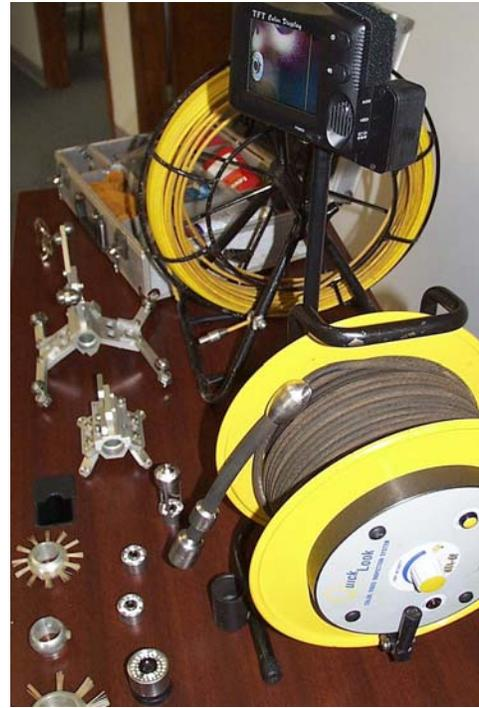
This system has been used successfully for the inspections verification after hydro-blast of power pressure piping. It has also been used for small item retrieval in oil lube lines of steam turbines.
